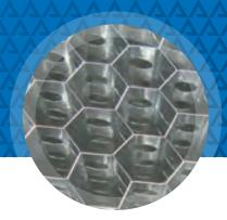
ARGOSY Vented (drilled) Aluminum Honeycomb Core is a stiff and stable lightweight product used primarily in tooling applications. Vented honeycomb facilitates the even distribution of heat through the tool. This ensures a consistent, even cure throughout the laminate and minimizes the risk of localized areas of semi-cured material.
