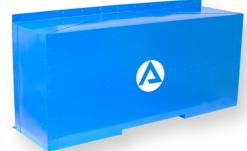
A complete testing procedure for certification of aluminum honeycomb is performed in-house according to Frontal Oblique and Small overlap Impact Crashworthiness Evaluation, NHTSA Test procedure, July 2015 and in accordance with the procedure defined in NHTSA TP-214D. The aluminum honeycomb blocks are processed such that the force deflection-curve when statically crushed is within the corridors defined for each of the 2 blocks.
